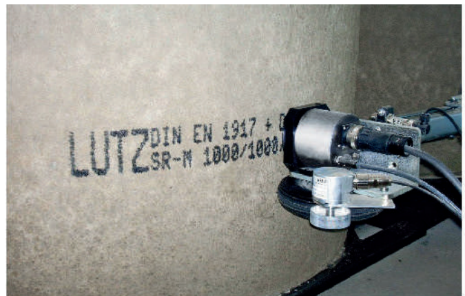
Marking of concrete pipes
